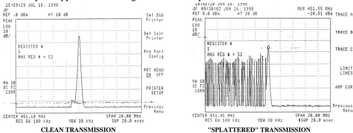
As the graphics so evidence, the spectrum analyzer is an excellent tool for detecting RF splatter. However, as stated earlier within this paper, the *Spectrum Analyzer* (SA) is an expensive piece of equipment if used solely for scanning and transmission screening purposes. The SA is also capable of performing a wide range of electronics related tests and functions.
